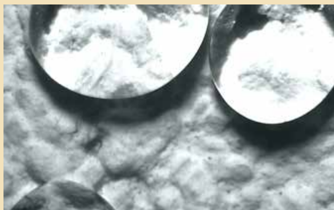
Compared to standard acrylic finishes (left), the AquaSol™ finish (right) creates a perfect spherical bead of water that repels off the surface, keeping it dryer and cleaner.
